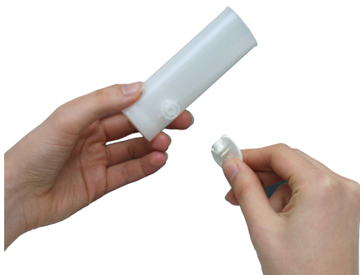
Figur: Montering af engangsflowtransducer_1
