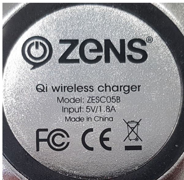
Figure: ZESC05B Qi wireless charger nameplate
